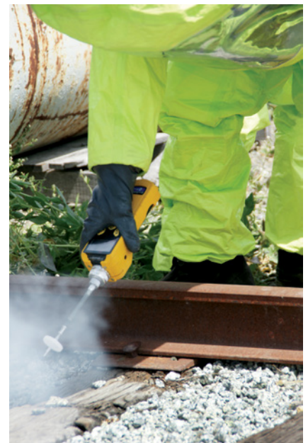
Workers can quickly measure VOCs and wirelessly transmit data via Bluetooth.
